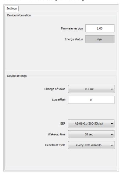
The device information shows the installed <u>Firmware version</u> and the current <u>Energy status</u> of the device is full charged or a battery is inserted. The Energy status must be **OK** to configure the device.
